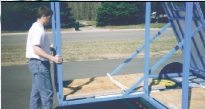
Slide battle station back and attach dolly wheels.
