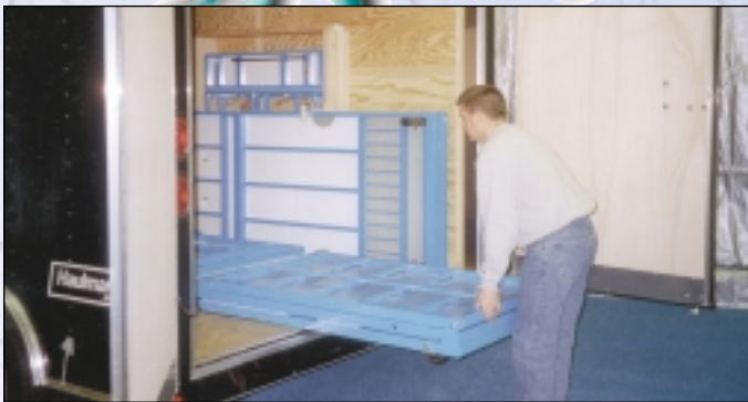
Lay unit down so it rests on its wheels, roll out of trailer and to set up location.
